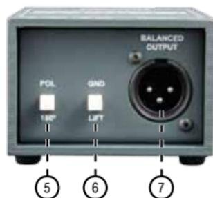
5. **POL:** Inverts the signal polarity by flipping pin-2 and pin-3 on the XLR output.
