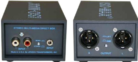
The Iso•Max DB-2MM is a stereo direct box designed to drive unbalanced hi-Z signals distances to 100 meters (300') or more at mic level without high frequency loss or introducing noise into the signal path.
