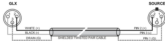
If your source device uses balanced 1/4" TRS connectors, you can use a balanced TRS to XLR adaptor cable wired as shown in the diagram below.
