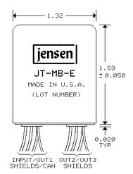
$\pm$ 26 AWG (7 $\times$ 34) UL STYLE 1061 COLOR CODED WIRE LEADS, 12" MINIMUM LENGTH
