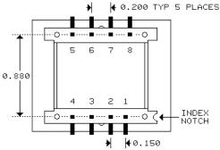
PIN NUMBERS NOT MARKED ON PART PINS ARE 0.025 SQUARE, 8 PLACES 0.040 DIA PC HOLES RECOMMENDED
