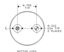
RECOMMENDED MOUNTING IS WITH VR-3 CLAMP (SUPPLIED WITH TRANSFORMER)
