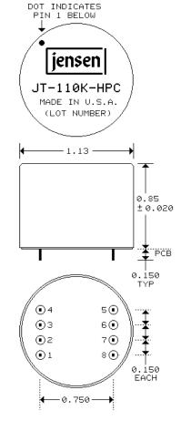
PIN NUMBERS NOT MARKED ON PART TERMINAL PINS 0.018 × 0.030 PC HOLES 0.040 DIA SUGGESTED
