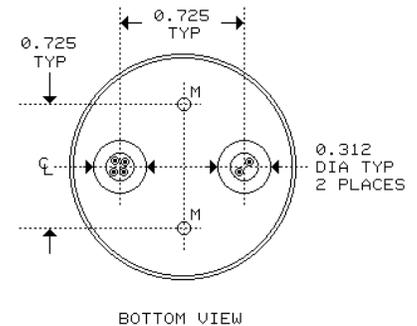
USE ONLY #4 TYPE B SELF TAPPING SCREWS IN HOLES "M". ALLOW NO MORE THAN 0.15" PENETRATION INTO TRANSFORMER HOUSING.
