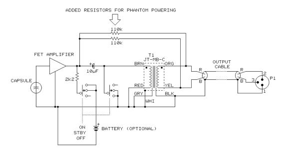
SCHEMATIC IS PER ORIGINAL, EXCEPT THAT RESISTORS ARE ADDED SO THAT +48 VOLT PHANTOM POWER CAN BE USED TO ELIMINATE BATTERY DRAIN. ALTHOUGH THE CIRCUIT WILL OPERATE OK WITHOUT A BATTERY IN PLACE, A GOOD BATTERY MAY BE KEPT INSTALLED AND THERE WILL BE NO DRAIN ON IT AS LONG AS PHANTOM POWER IS AVAILABLE. WITH A GOOD BATTERY INSTALLED, THIS MODIFICATION WILL NOT INTERFERE WITH NORMAL, NON-PHANTOM, OPERATION.
