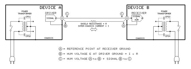
Figure 1 - THE HUM GENERATING MECHANISM The basic problem is that the shield is a common path for both inter-chassis "ground" <u>and</u> signal currents.
