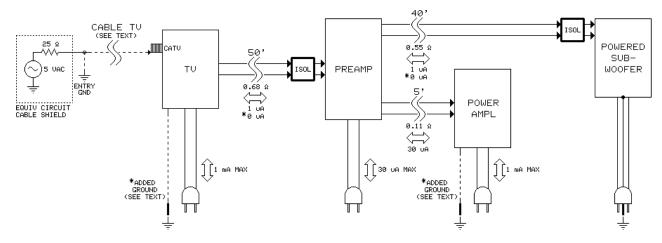
Figure 6 - THE EXAMPLE SYSTEM "AFTER"
