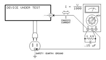
Figure 3 - MEASURING THE CHASSIS CURRENT
