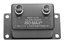
The Iso•Max VB-1BB is a single-channel 75  $\Omega$  video isolator for composite (baseband) video that is used to eliminate 60 cycle 'hum bars' even where ground voltage differences are very large such as in surveillance video systems, night clubs, video walls, broadcast stations, and industrial plants.
