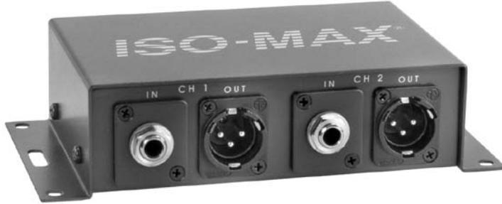
The Iso•Max DB-2PX is a stereo direct box designed to drive unbalanced instrument signals distances to 100 meters (300') or more without high frequency loss or introducing noise into the signal path.
